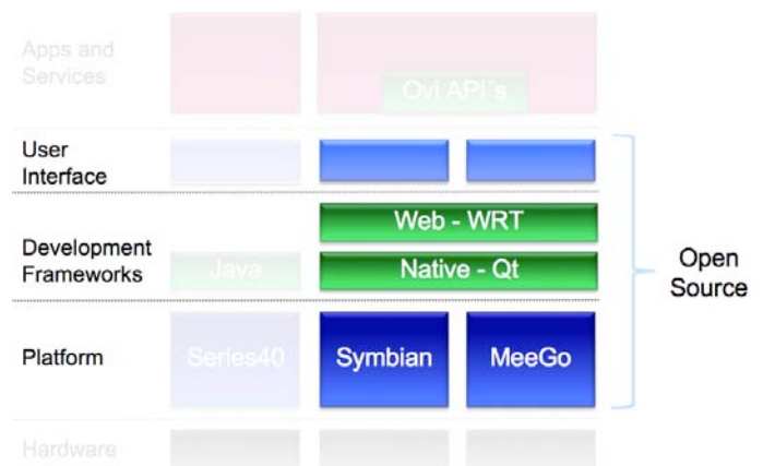
Figure 4 Open source components: Web Runtime (WRT) is based on WebKit; MeeGo is built from multiple open source projects; Qt and Symbian are open source projects.
