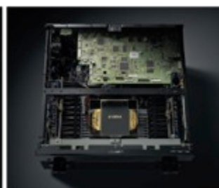
H-shaped Cross Member Frame and Symmetrical Power Amp Layout
