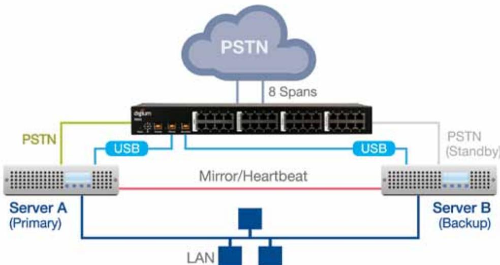
Under normal conditions the backup server (B) is synchronized with and monitors the health of the primary server (A) via the local area network. If the backup detects a hardware or software failure on the primary it will notify the R-Series to to redirect the PSTN connections and take over as the active system. Within seconds operations will resume with all services intact.
